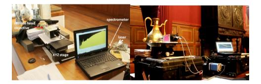
Figure 1: On-site Raman analysis using HE532 mobile set-up.
