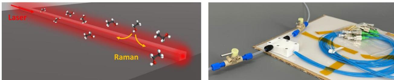
**Figure:** Schematic principle of WERS. A WERS sensor integrated in a flow cell for fluidic measurements.
