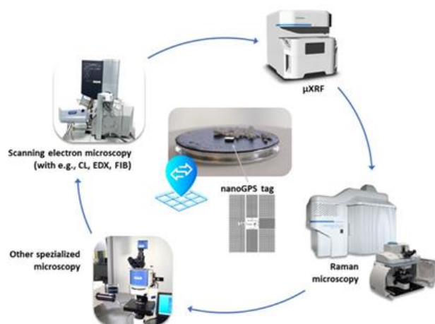
Figure 1: HORIBA's NanoGPS solution for POI relocation across SEM, \mu XRF, Raman, and other microscopy methods.
