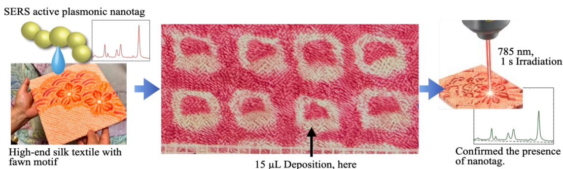
Figure 1: SERS based authentication with invisible plasmonic nanotag deposited on silk textile.
