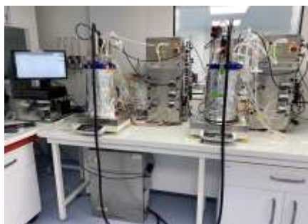
Figure 1: inline Raman spectrometer setup at pilot scale for biomanufacturing (CLIMBIN collaborative R&D project)
